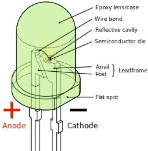
The anode (+ve) of the LED is connected to the longer leg. The cathode (-ve) as well as having a shorter leg, usually has a 'flat' on the corresponding side of the package.
