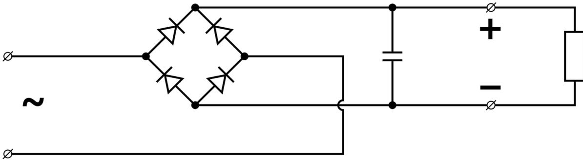
You can see in the following diagrams (if it's in colour!) that as the AC input alternates, the currents follow different paths so that the positive components always follow a path to the positive output, and likewise with the negative components:
