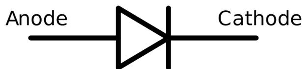
NOTE: for LEDs (Light Emitting Diodes) this voltage drop can be as high as 4.0V for blue/violet devices, and it is this that we call the *forward voltage* denoted  $V_f$ .
